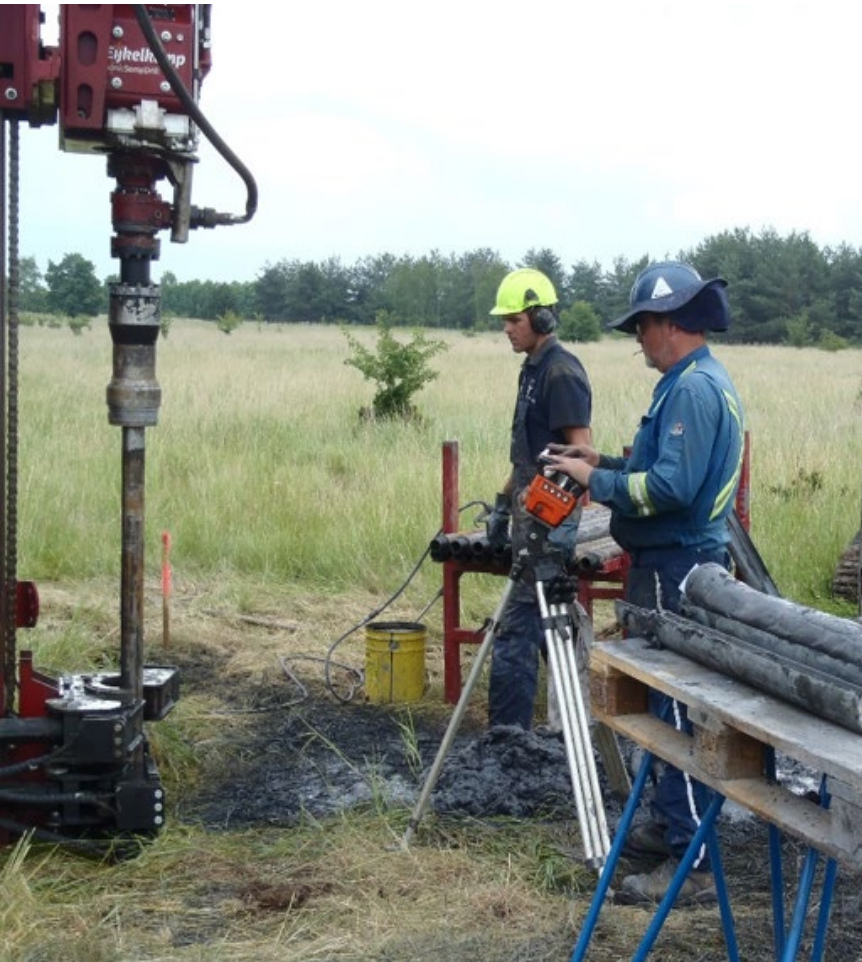
↑ Sonic drill – modern, effective sampling tool
