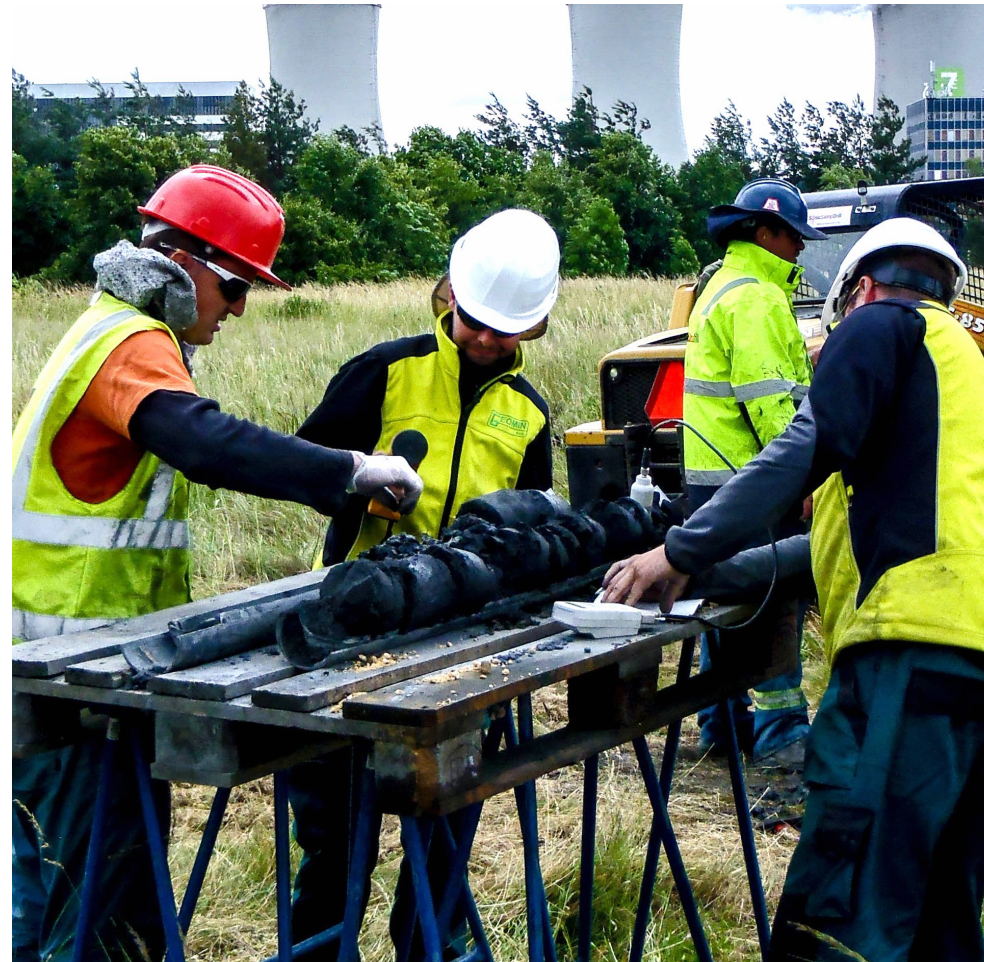
↑ Sonic drill “core” of soft, sandy tailings material
