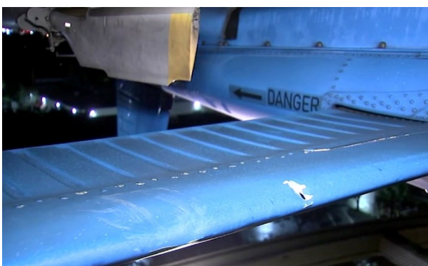
Image: The LA News Helicopter that was struck by a drone at 1,100 ft AGL. The closeup image shows puncture damage to the wing caused by the collision.
