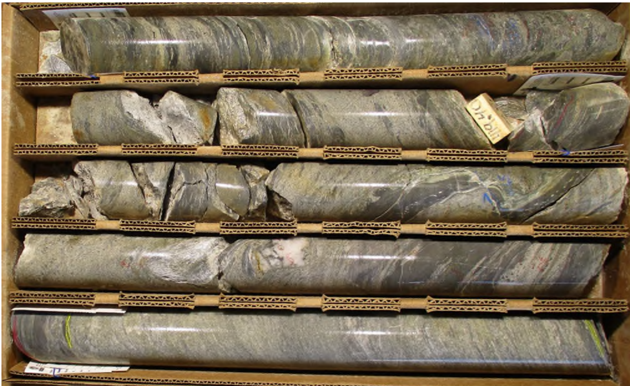
Figure 4: Massive sulphide mineralised interception at hole BMZ79 from 417.3m to 420.28m downhole depth. Sulphide mineralisation both follows cross-cut primary foliation in the hosting rhyolite rock. Sphalerite is pale brown; chalcopyrite bright yellow. Pyrite completes the visible sulphide assemblage
