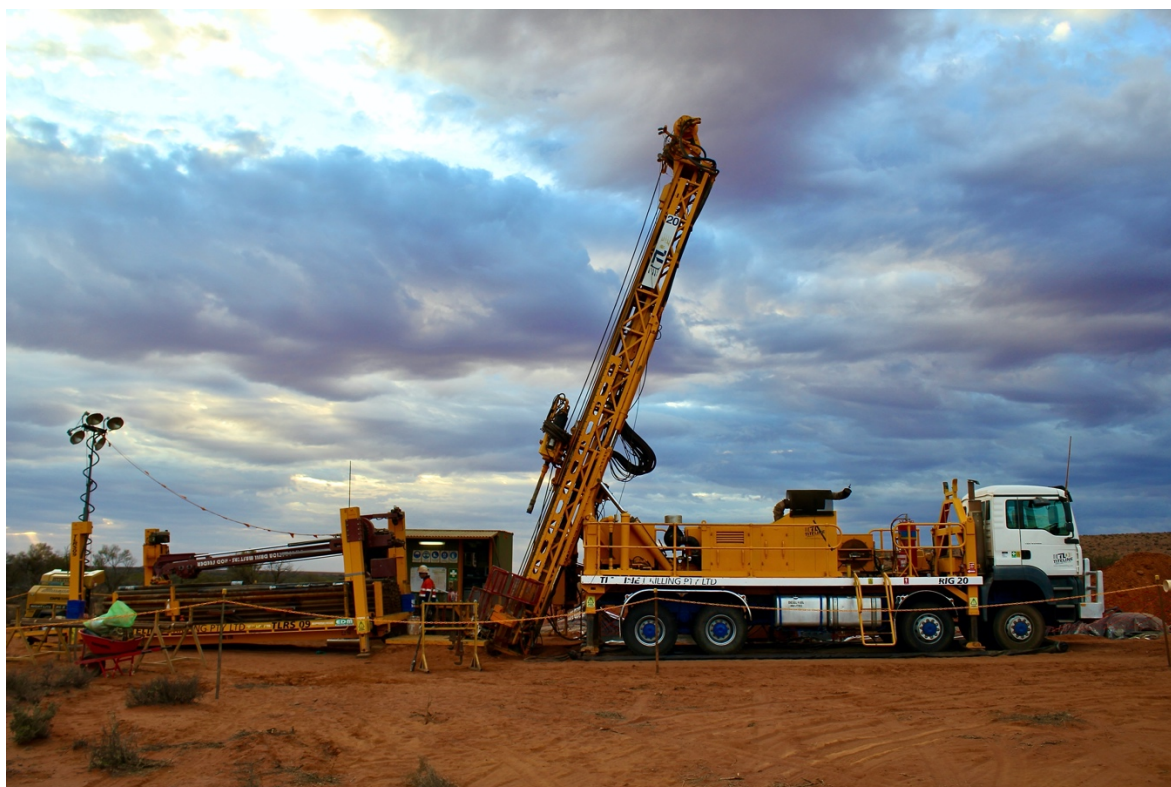
Photo 1: Titeline diamond drill set up on the first Maslins drill hole.
