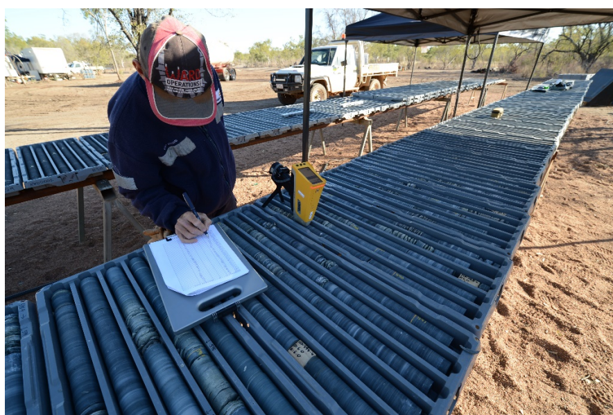
Figure 3. Logging of diamond drill core from the Nicholson West VTEM target.
