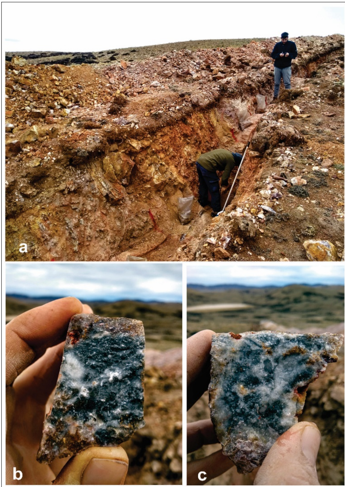
Figure 5 – 5A: Trench #3 displaying a 10 metre zone of quartz-sulphide breccia previously hidden from surface view by 30cm of recent volcanic ash. 5B and 5C: Quartz-sulphide breccia (assaying 5 g/t Gold) from diamond sawn channel sample in Trench #3. Sub-angular fragments of pyrite-arsenopyrite (blue-grey) within a matrix of chalcedonic quartz (white) which displays incipient banded texture.
