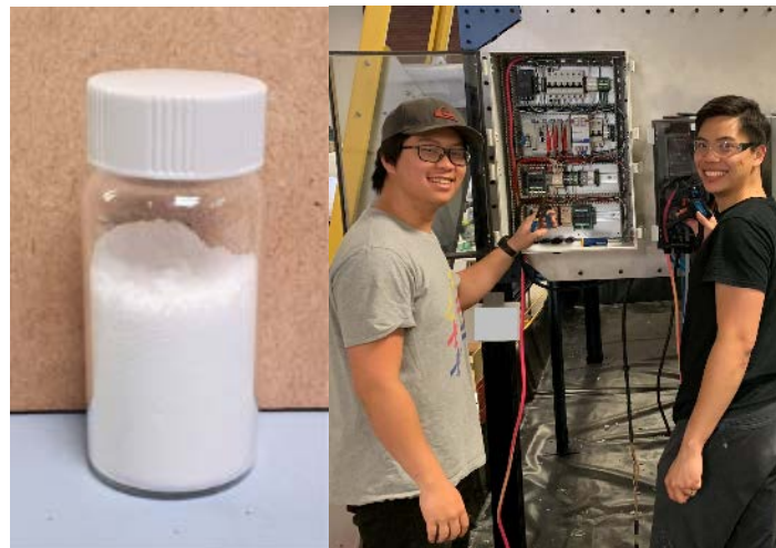
Figure 4: Lithium carbonate product with 99.9% purity and low impurities from the Kachi Lithium Brine Project using Lilac’s direct extraction ion exchange process. Pilot Plant under construction at Lilac’s facility in Oakland, California. Lilac materials engineer Garrett Lau (Ph.D. Northwestern University, B.S. Massachusetts Institute of Technology MIT) and process engineer Amos Indranada (B.S. University of California Berkeley) show the controls.
