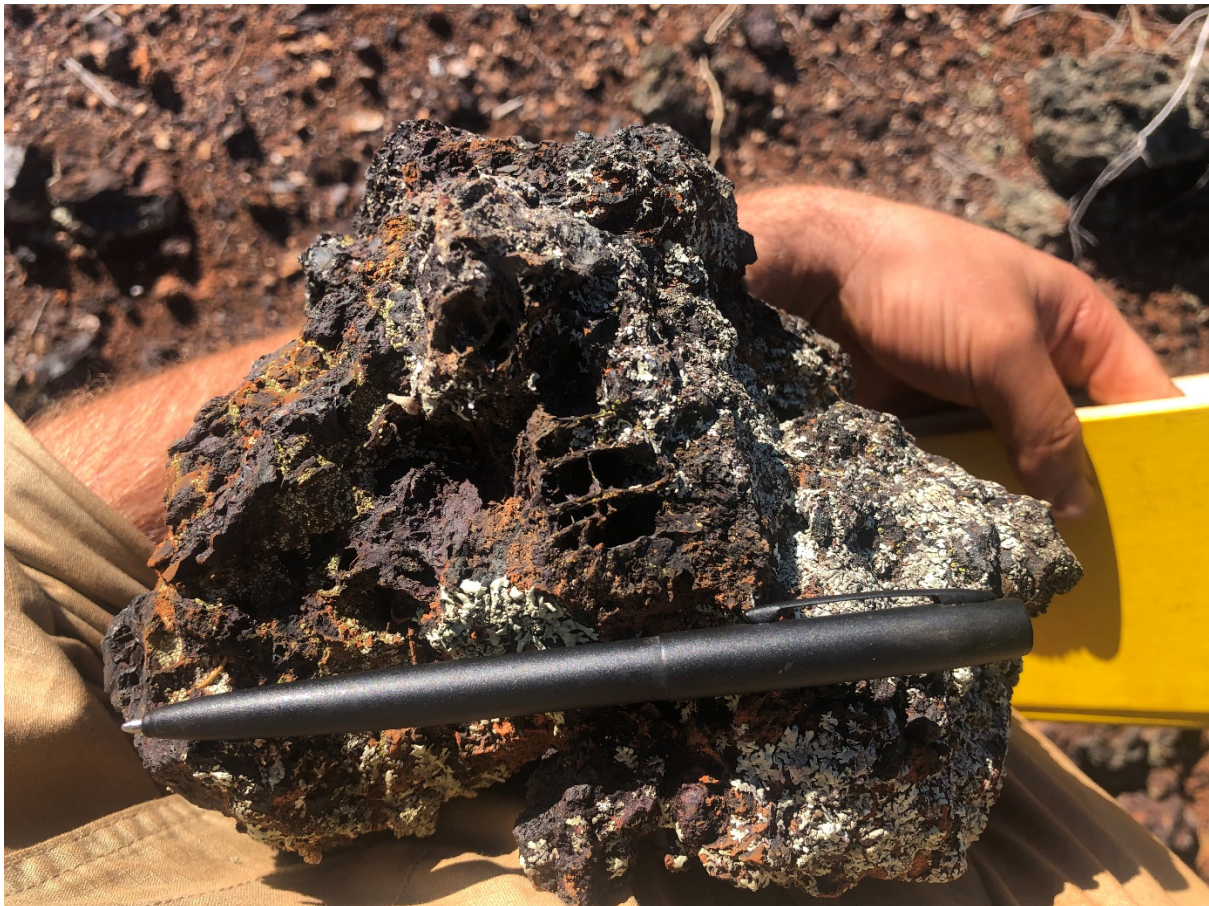
Figure 7: Gossan sample from Reindler’s Find showing box work textures after sulphides.
