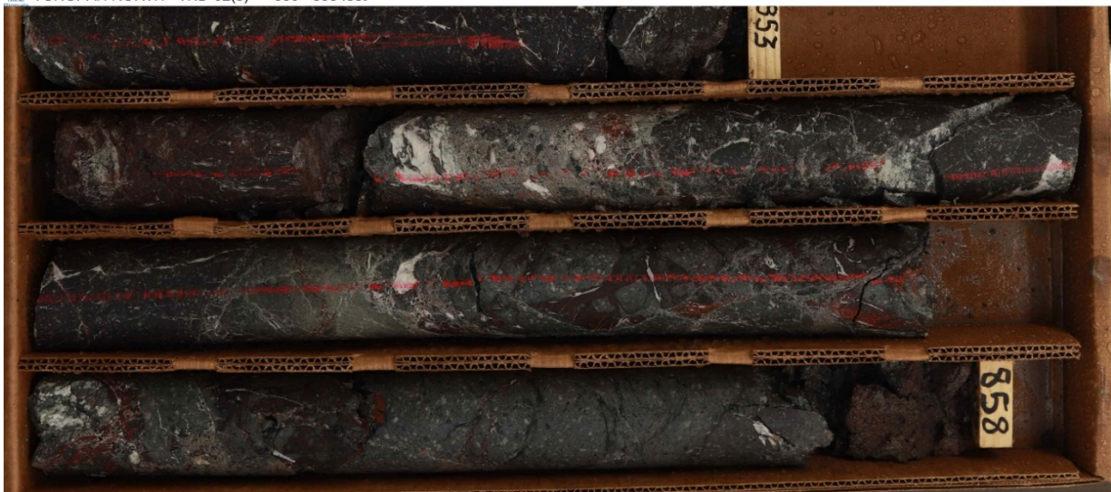
Figure 3. Photo of TND-02 Core showing mineralised interval from 260m (853ft) to 261.5m (858ft)
