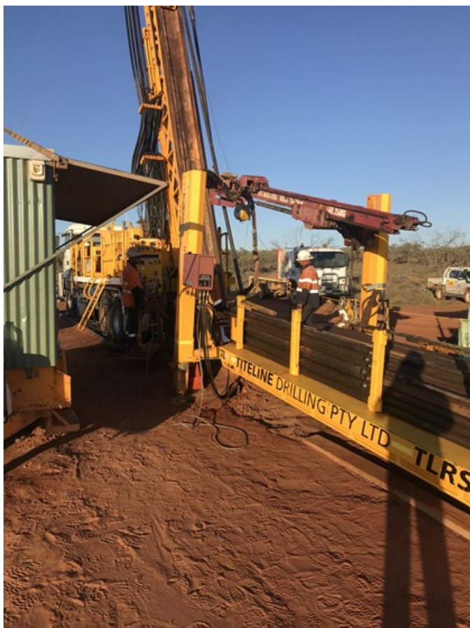
Photo 2: Titeline diamond drill rig set up on the first Maslins drill hole.
