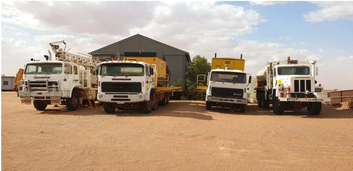
Figure 4: Drilling fleet ready for action during 2020. Comprising drilling rig, two compressor trucks with booster and 6x6 diesel fuel tanker.
