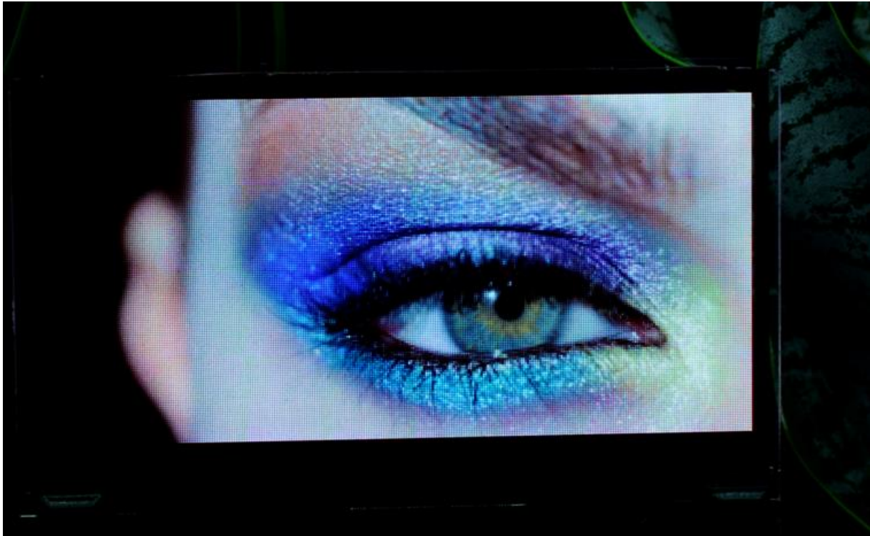
Image: X-Display (X-Celeprint subsidiary) microLED display prototype grown using BluGlass' RPCVD technology
