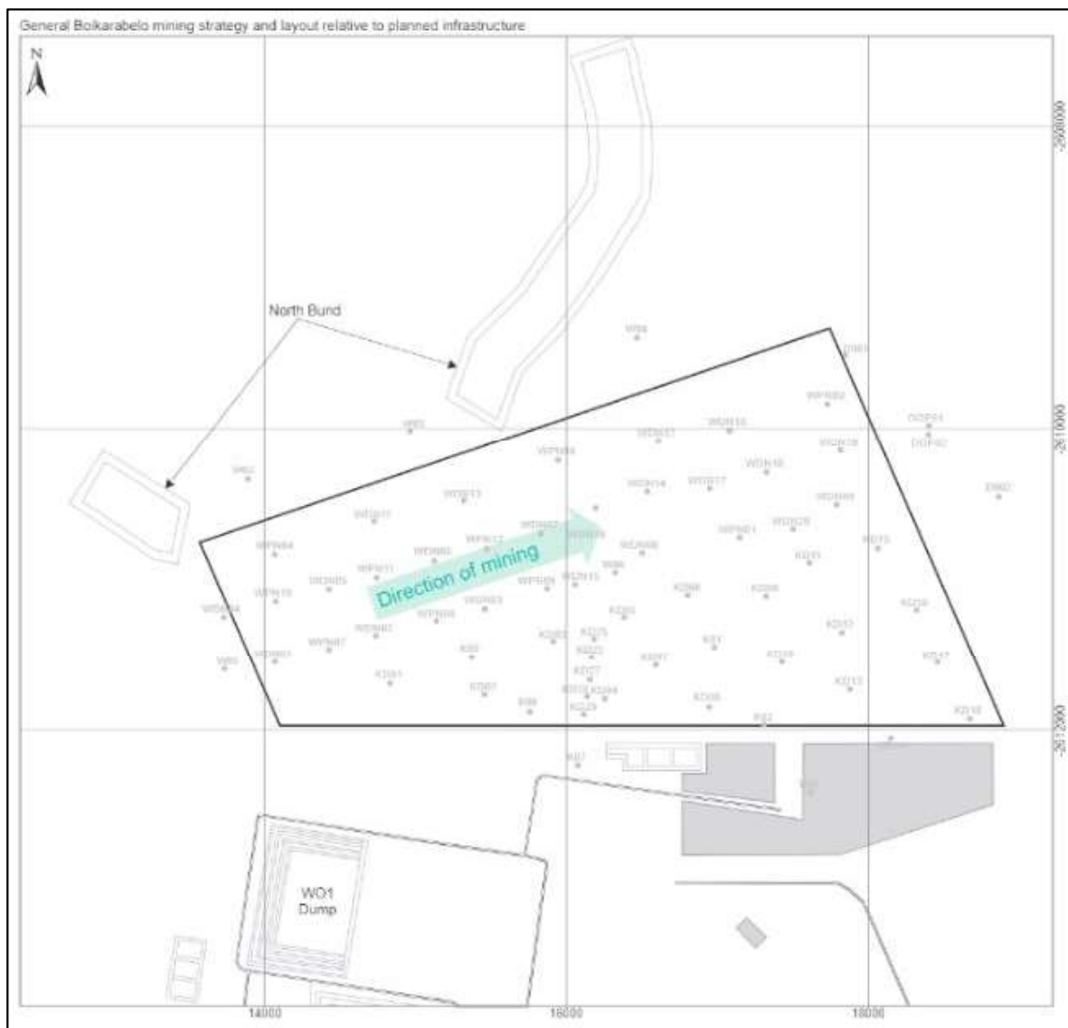
Figure 4-2: Mining area and infrastructure
