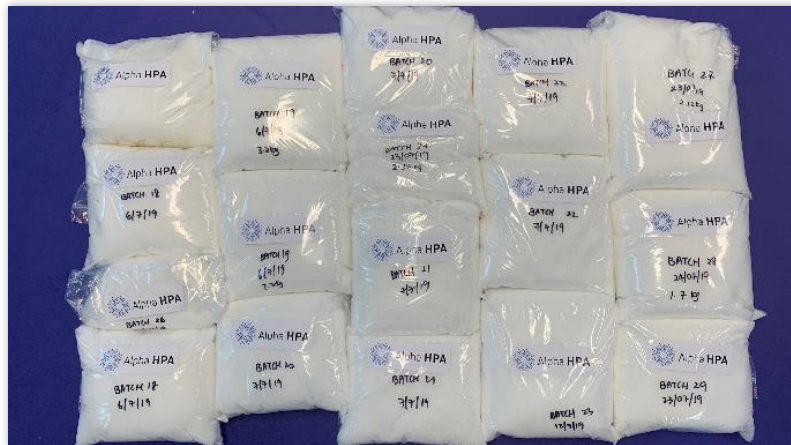
Figure 10: 21kg of high-purity aluminium salt, generated in the Pilot Plant over a 24 hour period
