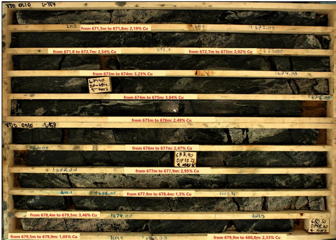
Figure 4: Drill core from hole VDD 213 showing massive chalcopyrite intervals.
