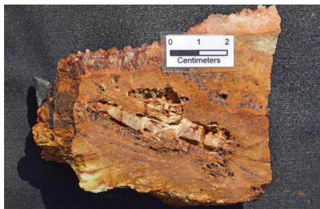
Photo 4: Outcrop sample KRS207444, 1.76g/t Au. Limonitic wallrock flooded by crystalline interlocking quartz, with a surface of crystalline prismatic quartz. Daeam Valley, Neungju Basin.
