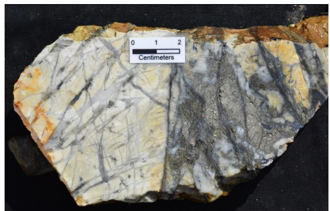
Photo 2: Float sample KRS207563 (from Central Quarry), 0.56g/t Au, 5.2% Pb, 2.79% Zn. Hydraulically brecciated, silica-illite-adularia altered rhyolite, with fine pyrite clasts, cut and flooded by chalcedonic quartz. Geum-Mar, Jinan Basin.
