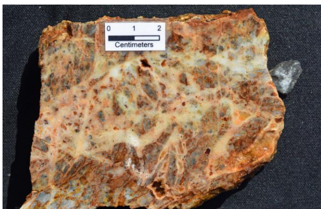
Photo 3: Float sample KRS207466, 3.16g/t Au, 2930ppm As. Hydraulic vein breccia, with limonite-haematite oxidised leucogranite clasts, set in a crystalline interlocking to mesocrystalline flood quartz matrix. Daeam Valley, Neungju Basin.
