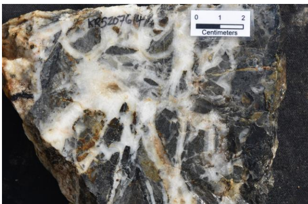
Photo 1: Float sample KRS207614, 1.93g/t Au. Hydraulic vein breccia, comprised of back carbonaceous siltstone, flooded by white chalcedonic to mesocrystalline quartz. Geum-Mar, Jinan Basin.
