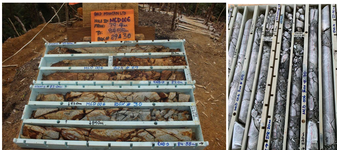
Figure 3. MCD006 –LHS strongly oxidised core from 79.4m to 84.5m with iron-oxides after sulphides, RHS core exhibiting intense fracturing and brecciation from 216.0m to 221.0m
