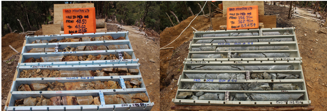
Figure 1. MCD005, Oxidised (LHS) and un-oxidised core from MCD005 exhibiting greater fracturing, veining and Alteration than MCD003 and MCD004
