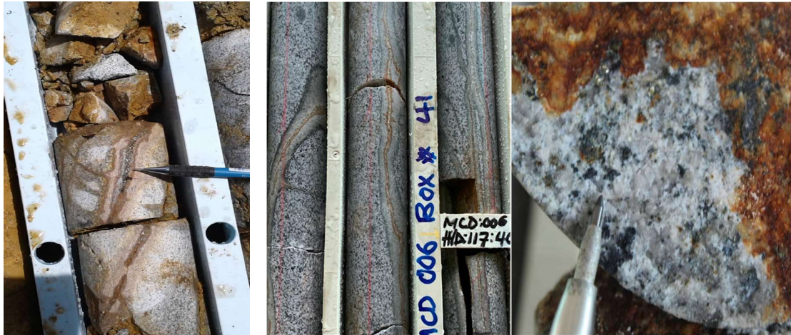
Figure 4. MCD006 – Quartz – pyrite veins with well-developed alteration selvages seen in MCD006, (LHS from 8.00m, contains approximately 5% sulphides, centre, veins 3mm wide with 5 mm wide alteration selvages , veins contain 30% pyrite and 70% quartz, with 2% pyrite in the tonalite matrix 115m to 117.60m, RHS – chalcocite (approximately 2%) on fracture surface associated with quartz and pyrite from 76m
