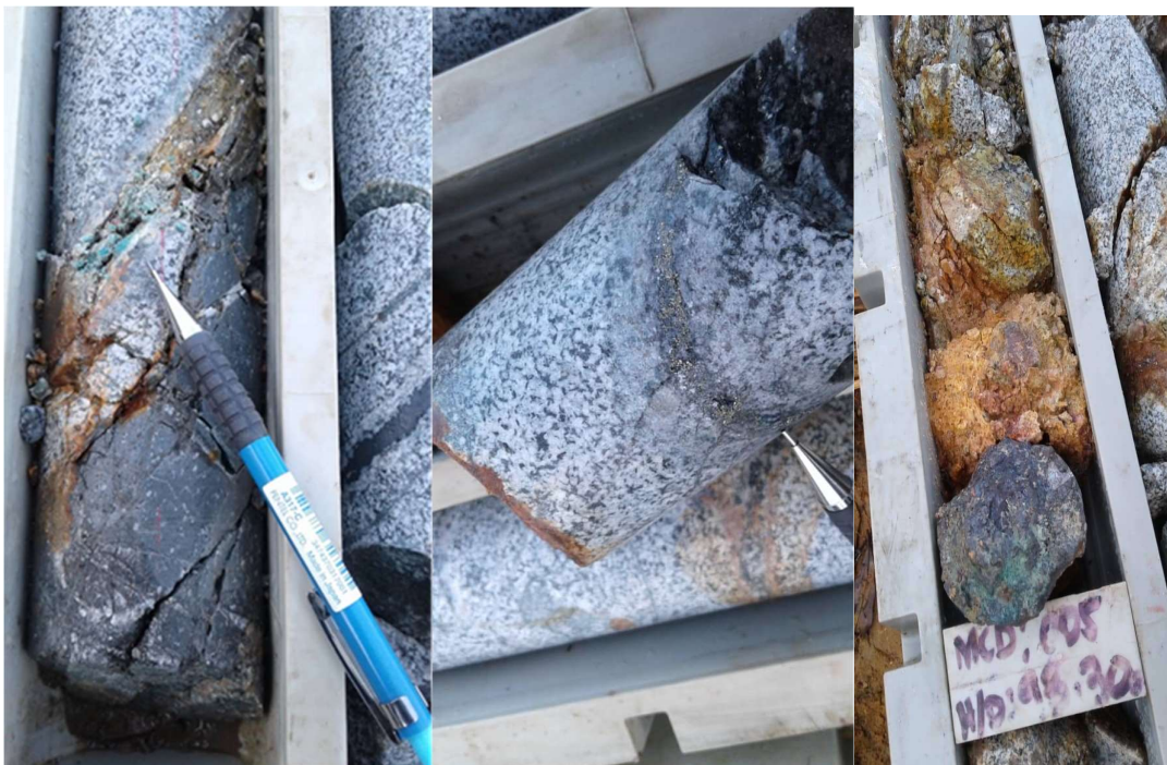
Figure 2. Examples of veining and mineralisation in MCD005, from left to right , qtz-pyrite-malachite bearing vein from 112.42m, vein is approximately 5mm wide and contains between 3 – 5% sulphide minerals, Centre , qtz-pyrite vein, which is 4mm wide with Fe-pyrite (5%) and molybdenum (0.5%) from 106.76m, Right , evidence of malachite and chalcocite coating on fracture surface at 98.30m, these copper minerals coat the fracture with the coating being 3mm thick
