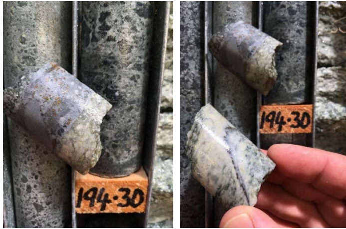
Figure 3: Magmatic vein breccias with copper mineralisation (chalcopyrite) and alteration selvages
