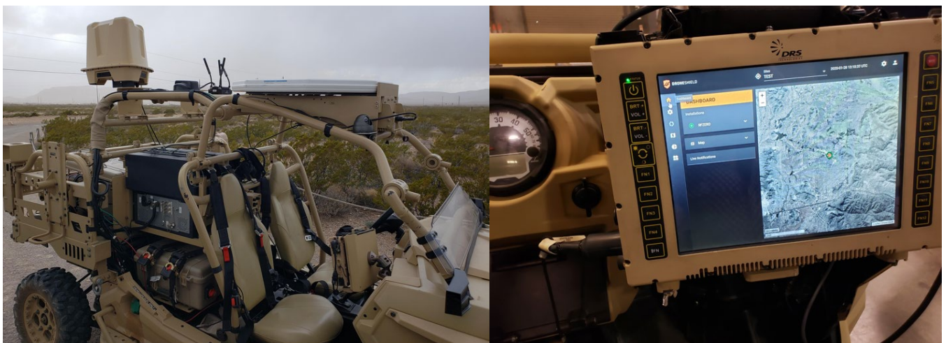
Image: DroneShield's RfZero™ counter-UAS system mounted on a Polaris MZRZ vehicle
