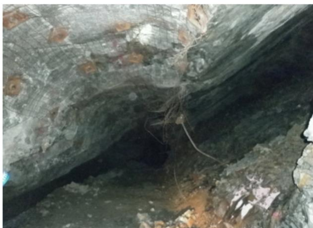
ABOVE: A mined area from Citigold's test mining showing the floor of the level drive, and the stope voids (ore extracted area) above and below the level. The ore has been cleanly extracted, showing how the mining method minimizes dilution by maintaining a narrow stoping 'slot' width.
