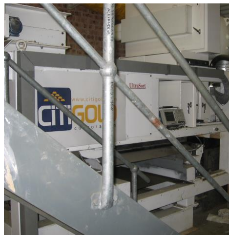
ABOVE: Charters Towers ore from Citigold test mining previously undergoing early-stage 'ore sorting' test trials. The aim is to mechanically remove unmineralised bulk rock 'dilution' that occurs in the ore mining process and reduce tonnage before it enters the wet end of the processing plant.
