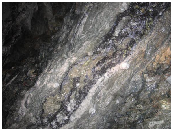
ABOVE: The gold ore at Charters Towers is visually very different to the host granite rock, and therefore relatively easy to follow for miners when excavating the tunnels in the ore in preparation for stoping (ore extraction).
