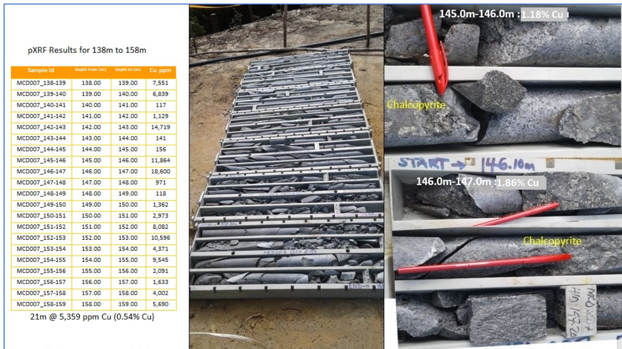
Figure 6. Core from MCD007 with averaged pXRF reading for each one-meter interval 4 . Mineralisation predominantly confined to fracture surfaces, with between 40 to 50% of the fractures in MCD007 coated with sulphides. The main sulphide mineral was iron-pyrite (~20%), followed by 1 to 2% chalcopyrite on the fractures 2 .
