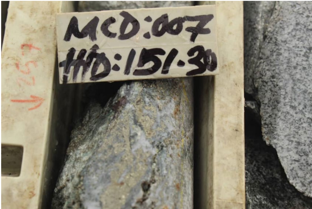
Figure 2. MCD007 – 100mm wide quartz - clay sulphide vein at 151.30m. Vein contains chalcopyrite (~5%), pyrite (~10%) and molybdenum (~0.5%).
