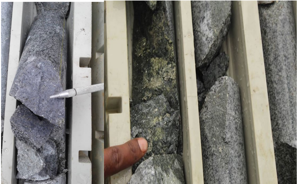
Figure 3. MCD007 – Mineralisation Styles. (LHS) 203.20m - Molybdenum covers the entire fracture surface. (RHS) from 146.20m, fracture coated with iron pyrite (~40%) and chalcopyrite (~5%) 2 . Layer of sulphides on fracture is ~2mm thick.
