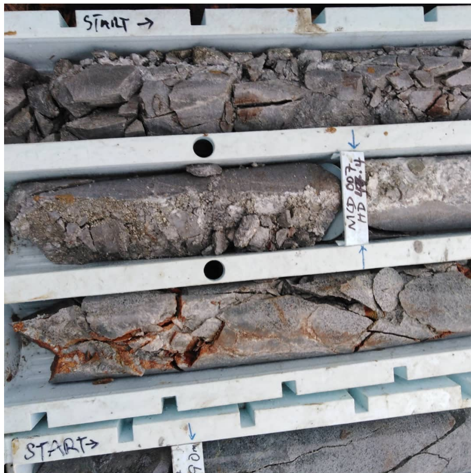
Figure 4. MCD007 – Strongly fractured and clay pyrite altered core from 46m to 47.40m Pyrite content in clay between 47.00m to 47.44m is approximately 10% 2 .
