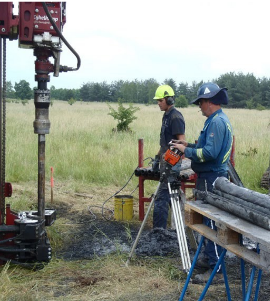
Sonic drill – modern, effective sampling tool
