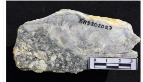
Polyphasic hydraulic vein breccia with rip-up vein fragments and a central black sulfidic band comprised of fine-grained pyrite & sulfosalts.
