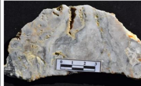
Polyphasic, crudely banded mesocrystalline grey-white quartz vein with localised ghosted quartz pseudomorphs after bladed calcite & wisps of bluish-grey sulfides & sulfosalts.
