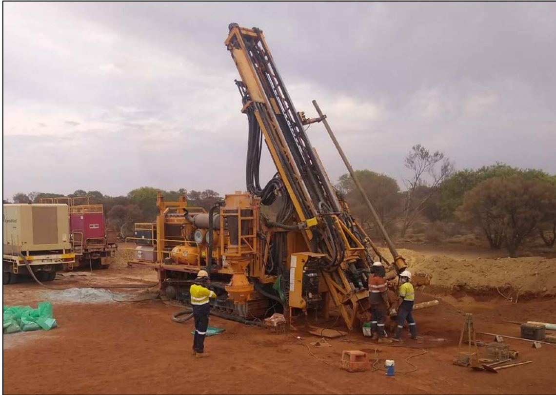
Image 1: Reverse Circulation (RC) drilling at Marymia
