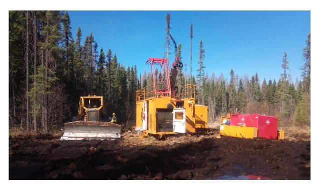
Figure 1 - Orbit -Garant Diamond Drill Rig setting up on hole AUDD0001 within the Pickle Crow tenement areas in Ontario, Canada.
