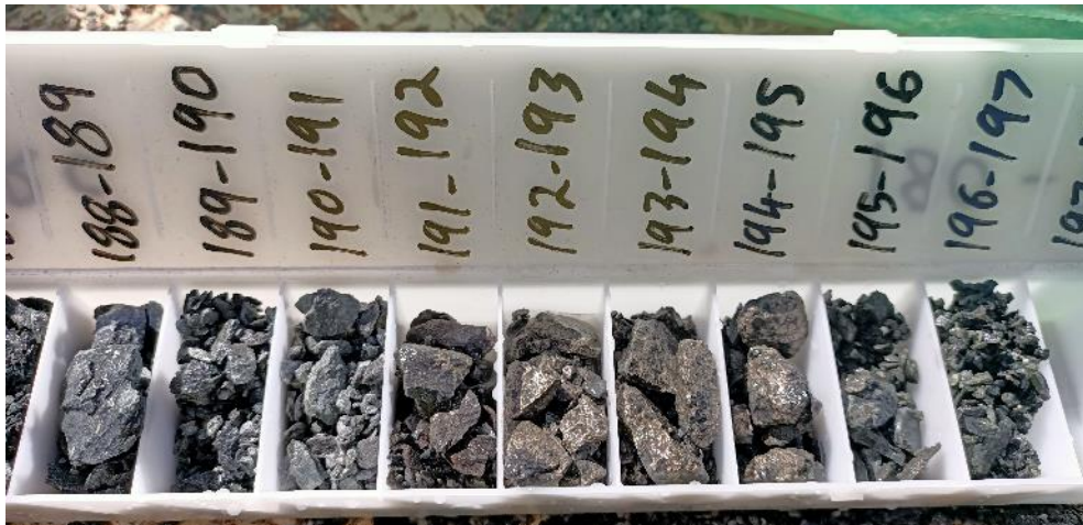
20RVRC043 (from 191m – 3m of massive sulphides - dominantly pyrite)
