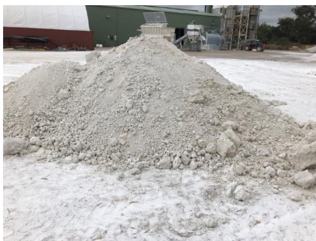
Figure 8 – Raw kaolinized granite, after auger sampling. The visible lumps are easily broken by hand
