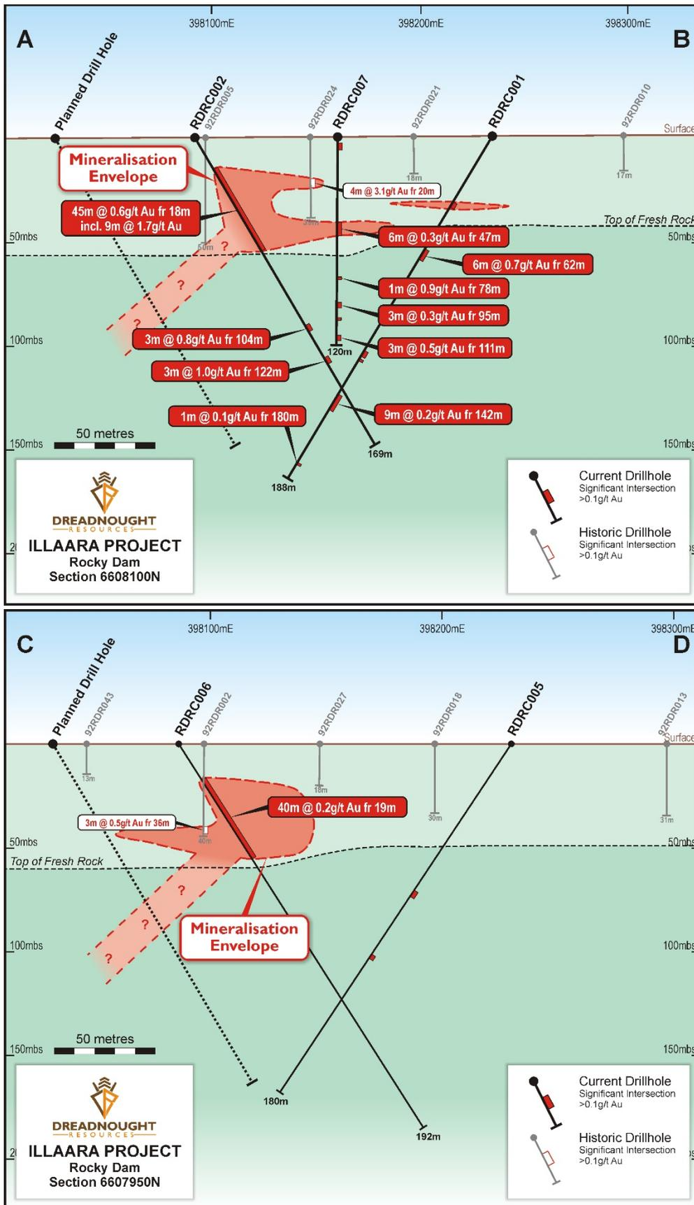
**Figure 2: Cross section through CRA-North showing thick shallow mineralisation in the oxidised bed rock, the interpreted lode dipping off to the west and planned follow up drilling**
