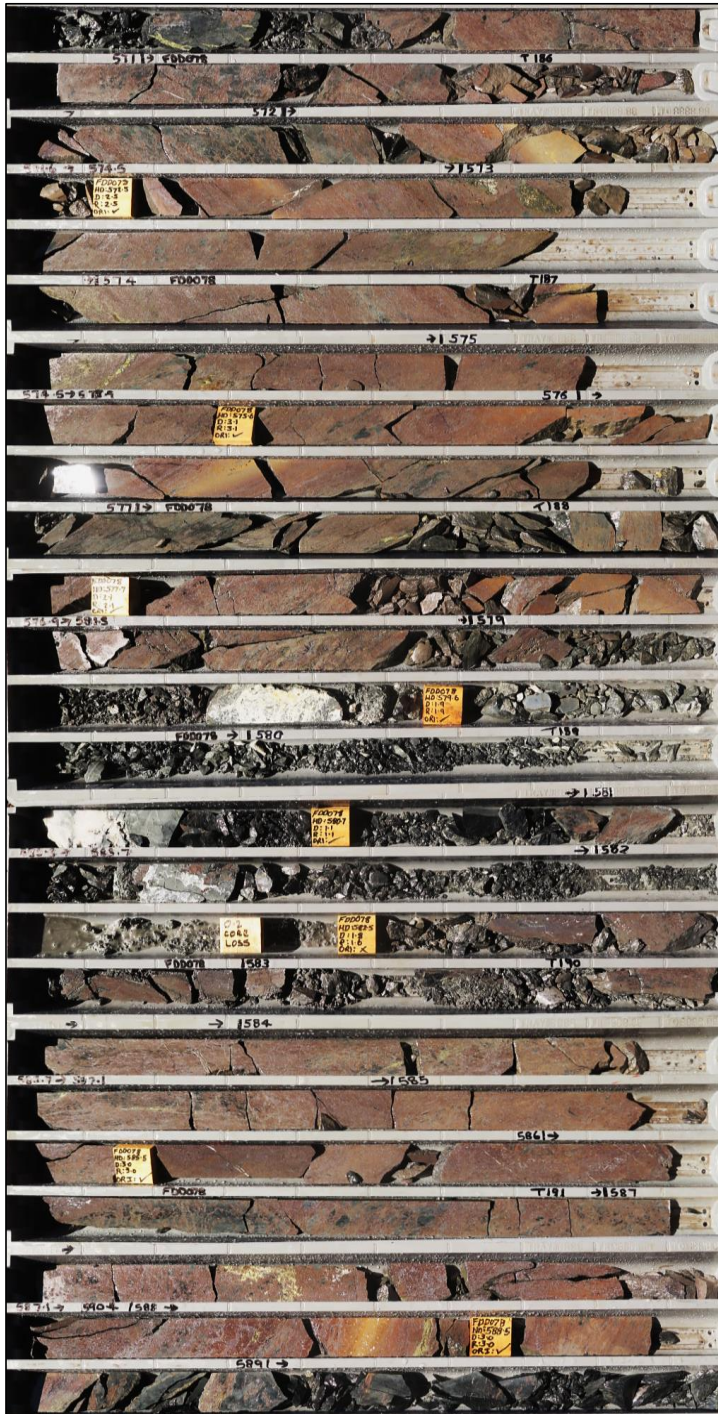
Figure 4: Cut diamond drill core from hole FDD078 at Federation, showing sphalerite-dominant massive and semi-massive sulphides (light brown) over a 22 metre interval
