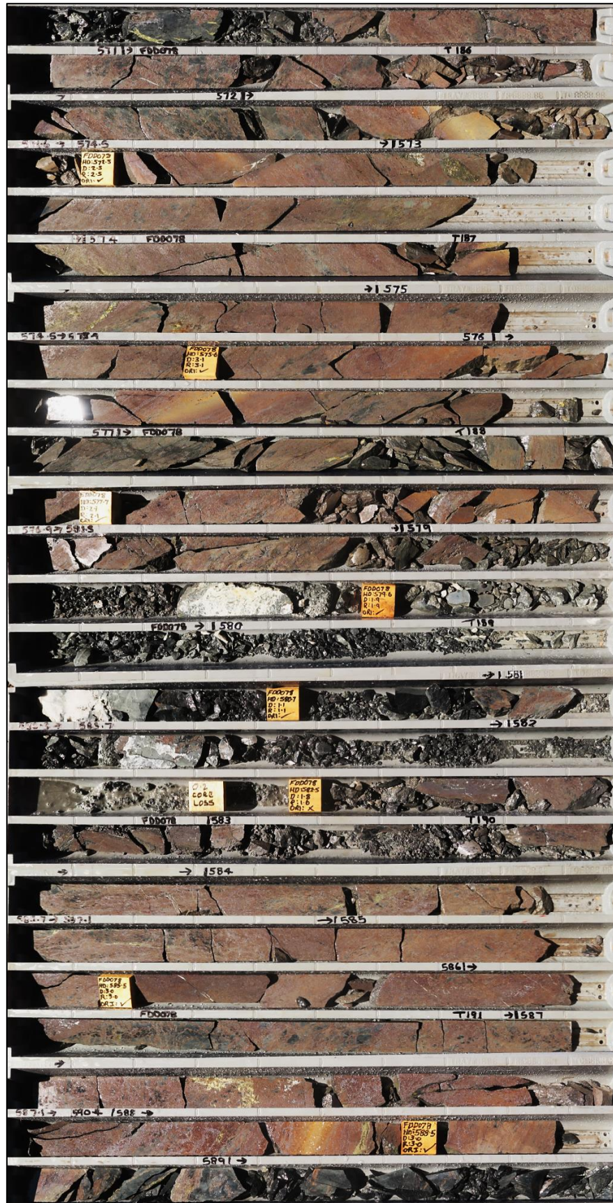
Figure 4: Cut diamond drill core from hole FDD078 at Federation, showing sphalerite-dominant massive and semi-massive sulphides (light brown) over a 22 metre interval
