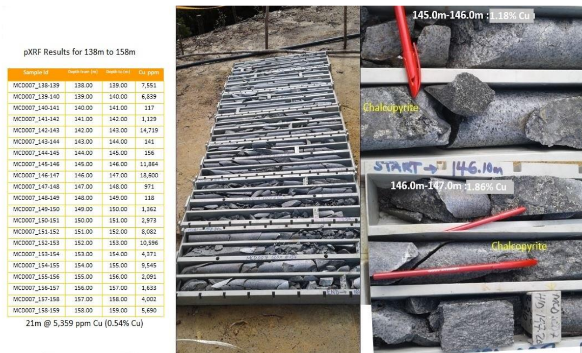
Figure 4. Core from MCD007 with averaged pXRF reading for each one-meter interval 2 . Mineralisation predominantly confined to fracture surfaces, with between 40 to 50% of the fractures in MCD007 coated with sulphides. The main sulphide mineral was iron-pyrite (~20%), followed by 1 to 2% chalcopyrite on the fractures 2 .
