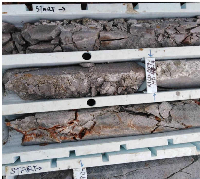
Figure 3. MCD007 – Strongly fractured and clay pyrite altered core from 46m to 47.40m Pyrite content in clay between 47.00m to 47.440m is approximately 10%
