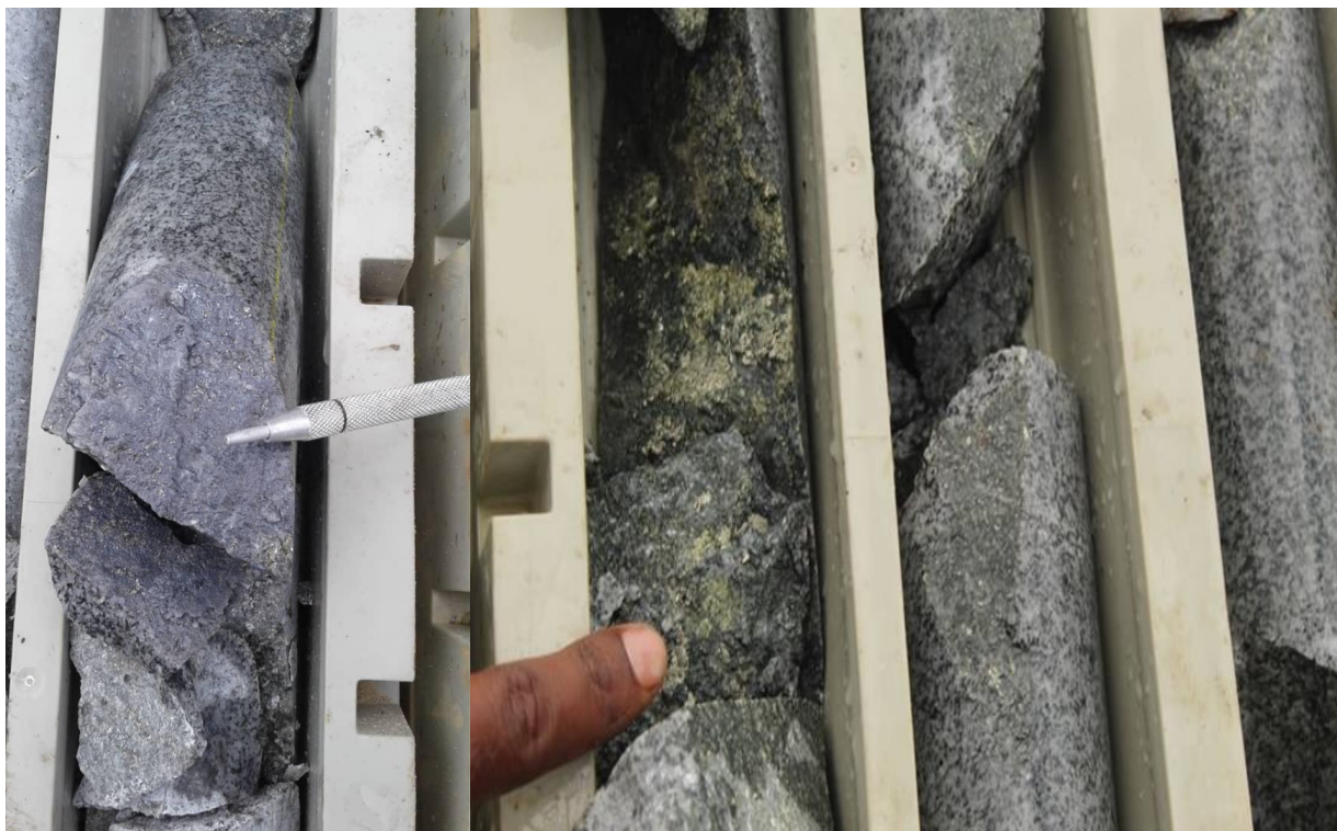
Figure 2. MCD007 – Mineralisation Styles. (LHS) 203.20m - Molybdenum covers the entire fracture surface. (RHS) from 146.20m, fracture coated with iron pyrite (~40%) and chalcopyrite (~5%) 2 . Layer of sulphides on fracture is ~2mm thick.
