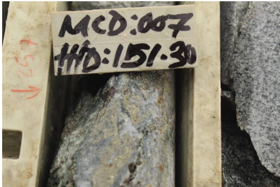
Figure 1. MCD007 – 100mm wide Quartz - Clay sulphide vein at 151.30m, vein contains chalcopyrite (5%), pyrite 10% and molybdenum (0.5%)
