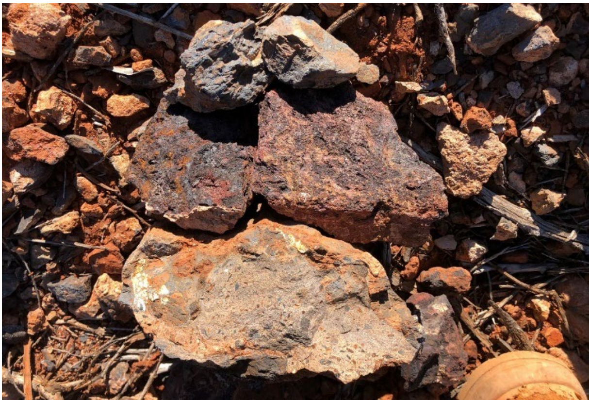
Figure 7: Rock Chips from EZ Hill (220729E, 6752781N UTMz51) showing black shale on top, gossan in the middle and felsic volcanoclastics on the bottom.
