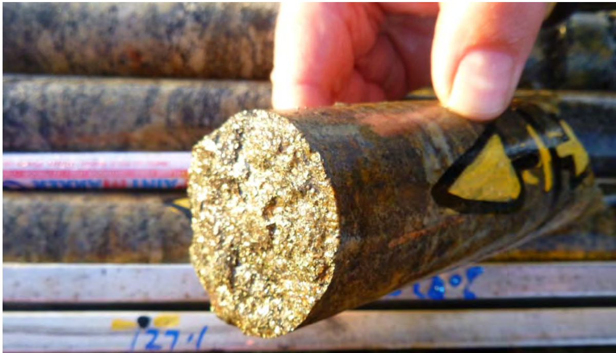
Figure 10: An example of the strongly pyritic bands in albitic gneiss in DD95STV3
