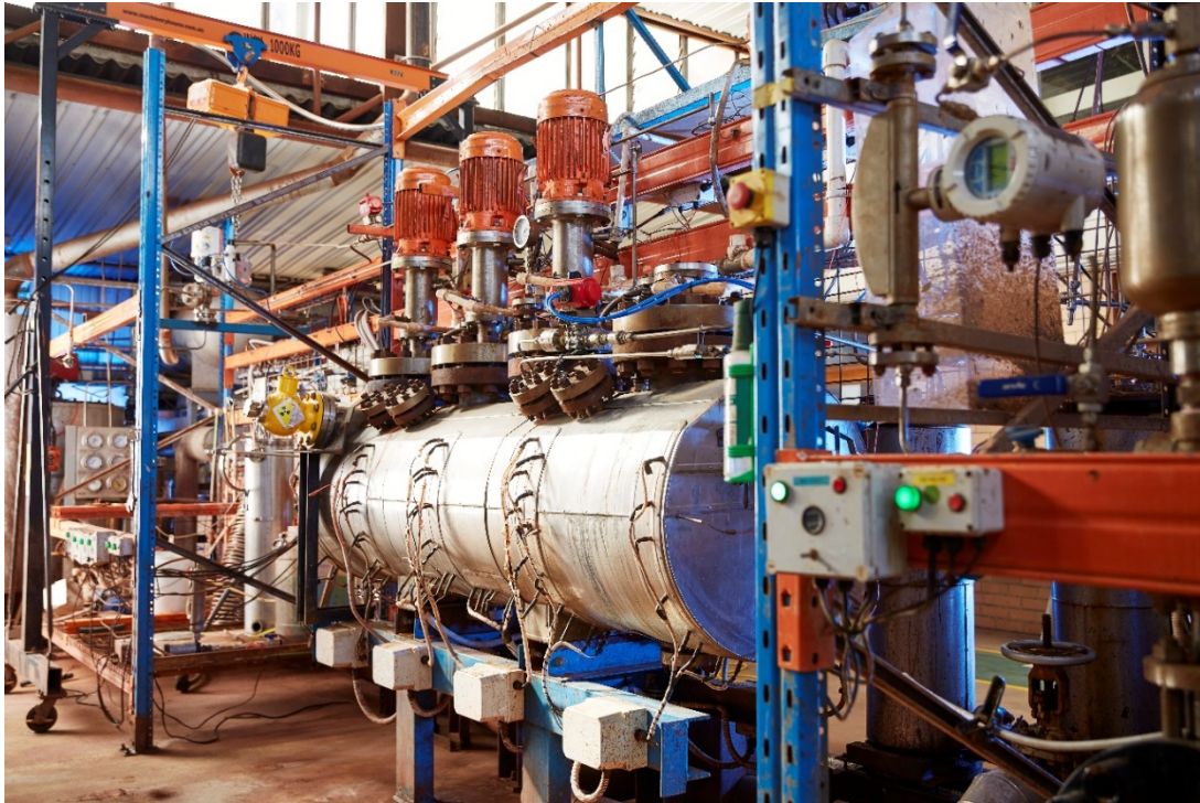
Figure 3: The autoclave at Australian Mines' demonstration plant. Cobalt-nickel-scandium rich slurry is heated to 250°C at 40 atmosphere pressure and mixed with sulphuric acid inside a titanium-lined autoclave vessel to quickly and efficiently leach the nickel, cobalt and scandium into solution.
