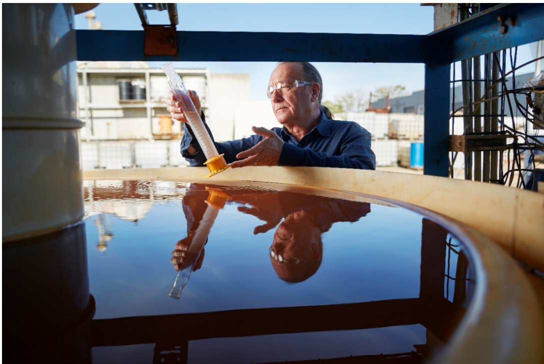
Figure 2: Sampling of the thickener overflow at Australian Mines' demonstration plant. The thickener is the final stage of the beneficiation plant after screening, crushing and grinding of the Sconi ore. The thickener underflow is pumped to the slurry storage tank ahead of being fed into the autoclave.
