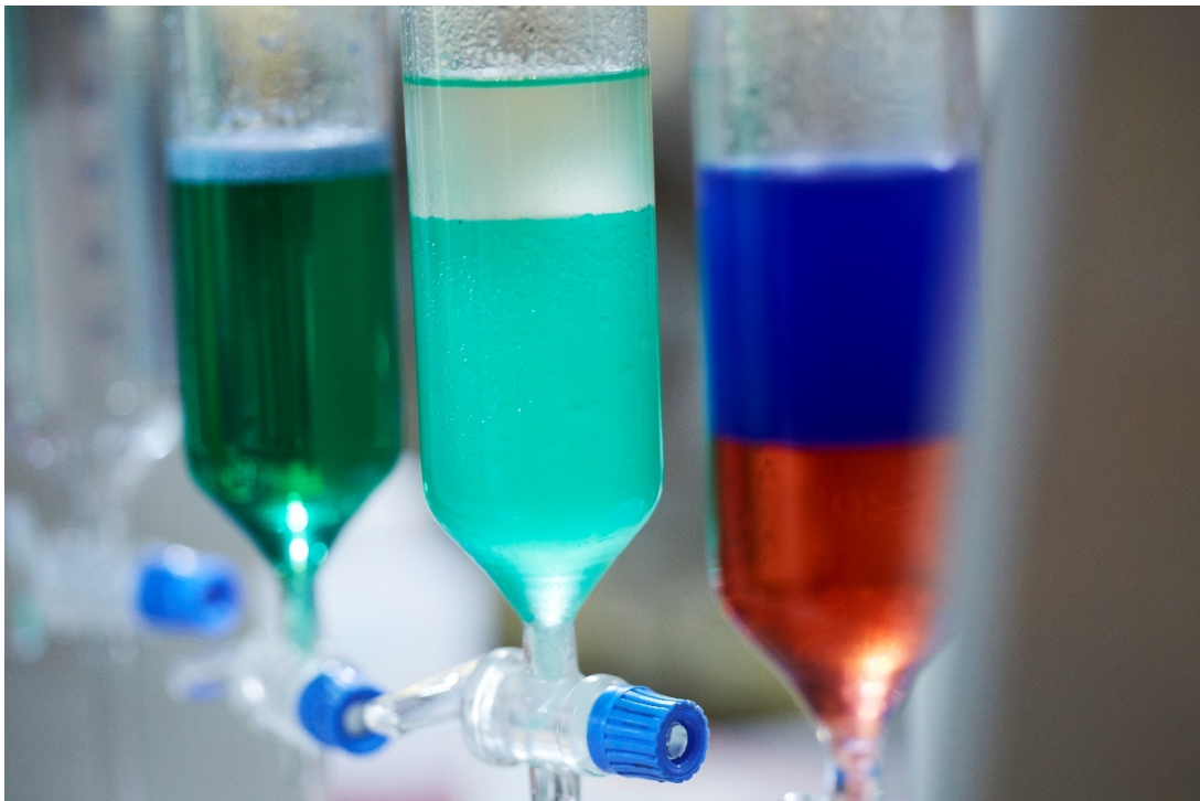
Figure 4: Laboratory example, taken at Australian Mines' demonstration plant, of the separation and purification of nickel sulphate and cobalt sulphate using solvent extraction and ion exchange.
