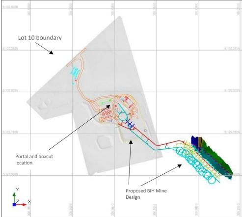
Figure 1: Plan view of Bird In Hand mine workings.
