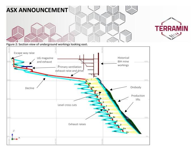
The proposed mining method for extraction of the Ore Reserves is Jumbo cut and fill, mining top-down with 20m level intervals mined in four lifts or flitches. The first is a driving flitch, the second a floor strip and the final two are back strips. Backfilling of the first two flitches will be by cemented rock fill with the top two flitches on each level being loose rock filled.
