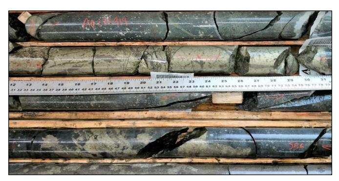
Core from the 4.1m zone of mineralisation hosted in Feldspar Porphyry (black and white speckled core) assaying 5.3% Cu, 4.9g/t Pd, 0.9g/t Pt, 0.26% Ni, 12g/t Ag from 55.3m in ZA-19-05 (including the 0.5m bonanza grade zone above the tape measure).
