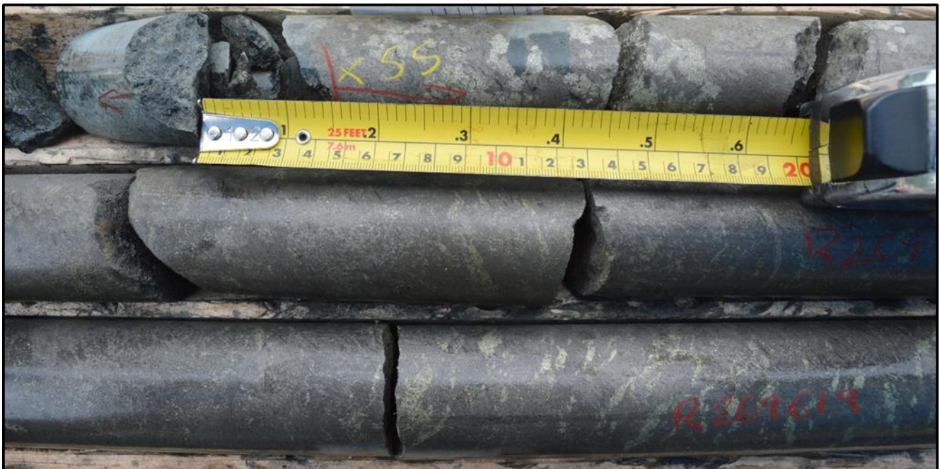
Figure 1: ZA-20-04. Mineralised gabbro (net-textured sulphides) in contact with massive sulphide (pyrrhotite with chalcopyrite and pyrite) at 55m downhole.
