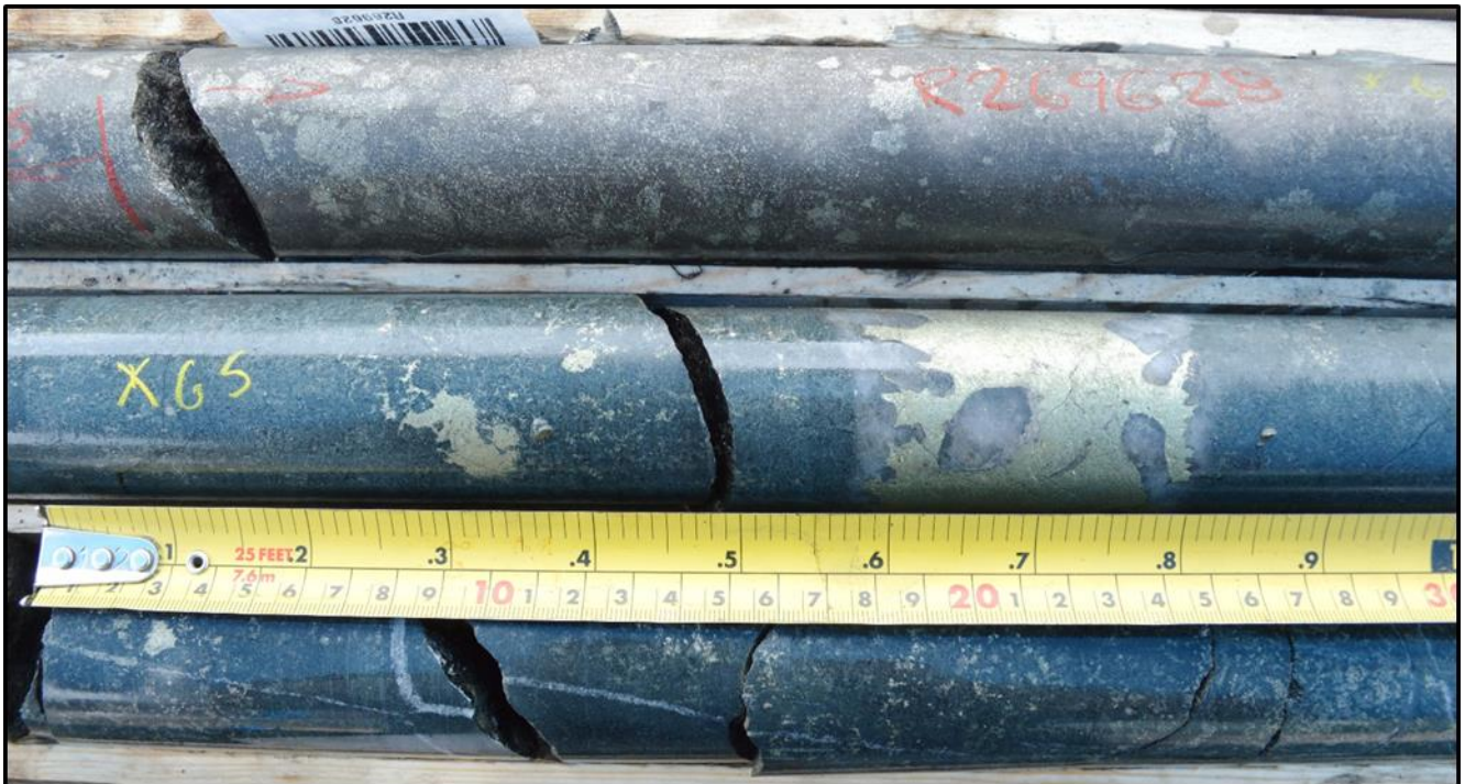
Figure 2: ZA-20-04. Massive sulphide (pyrrhotite with coarse pyrite blebs) at 65m downhole in contact with mineralised gabbro containing massive chalcopyrite.
