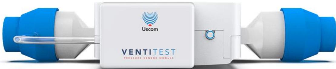
VentiTest is a multi-path ultrasonic ventilator test device with PC based display and analytics designed for pressure, flow and volume testing and calibration of ventilator outputs.
