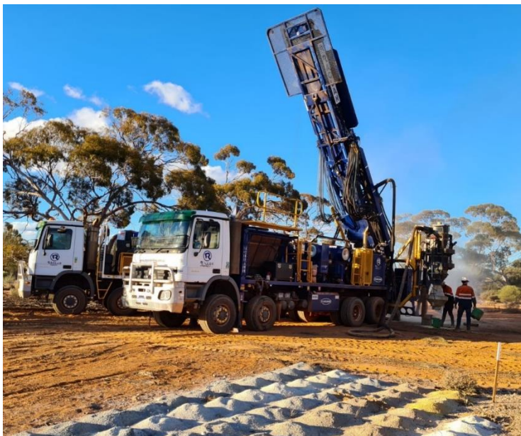
Figure 1: RC rig drilling hole RDRC008 at CRA-North
