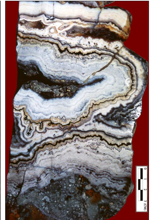
Cut slab of Lighthouse Vein, colloform banded epithermal Au-Ag
