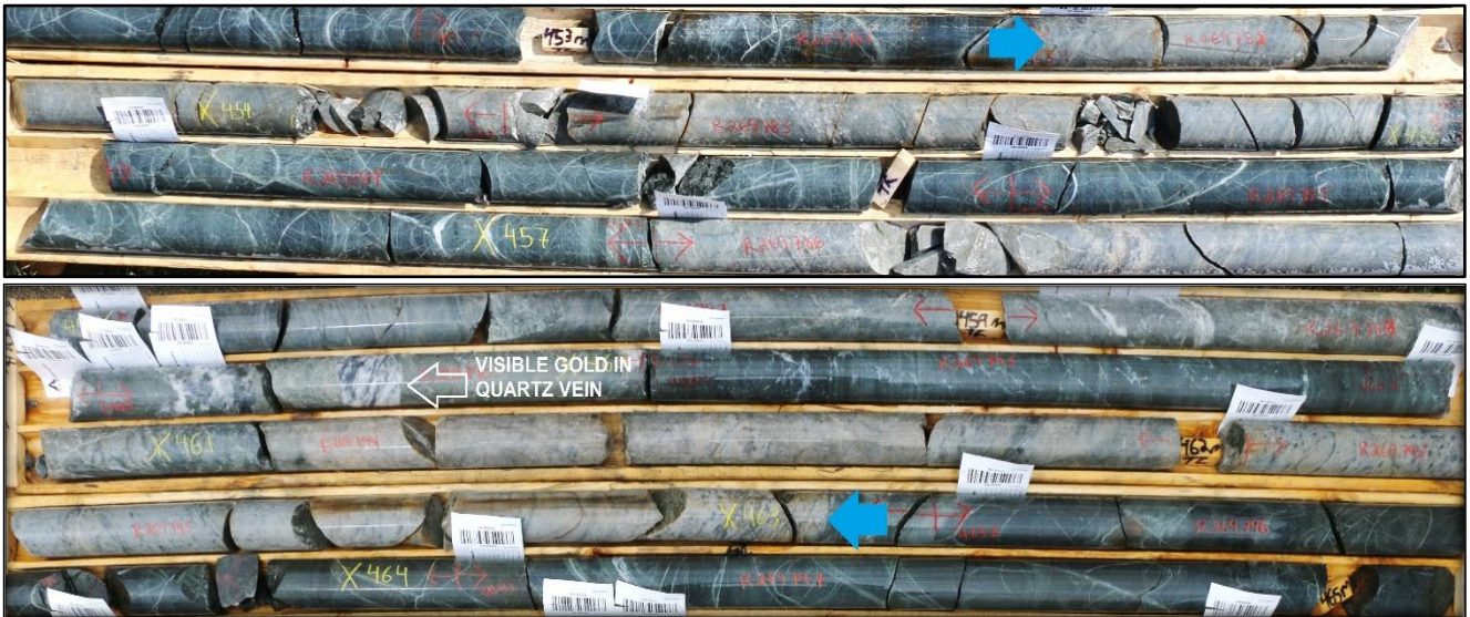
Figure 8: Very fine grained visible gold in quartz vein at ~459.8m downhole occurs within an intermittent ~10m wide (marked by blue arrows) strong silica-carbonate alteration zone with fine grained pyrite from 453.4 to 456.1m; 457.2 to 460.1m; 461.1 to 463.1m downhole (ASX 9 and 14 July).
