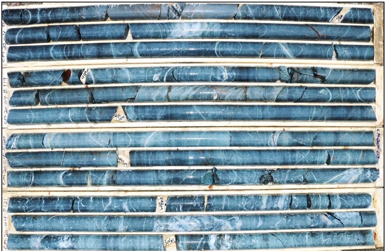
Figure1: Hole CM-20-04. This image shows an approximate 16m downhole portion of ~ 20m of mostly altered footwall rocks exhibiting silica-carbonate veining and breccias from ~480.3m to ~501.3m.
