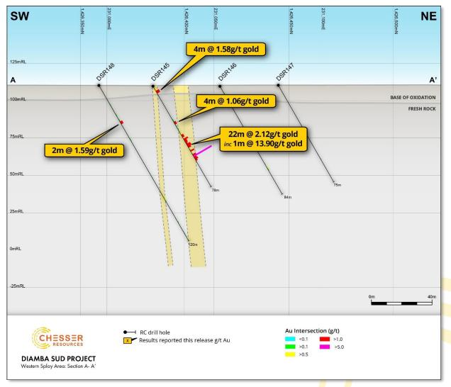
Figure 2: Section A-A' looking northwest, showing approximately 11m true width main mineralised zone with narrow footwall structure. Mineralisation is hosted in brecciated carbonates, with quartz and pyrite infill and strong albite-hematite alteration.
