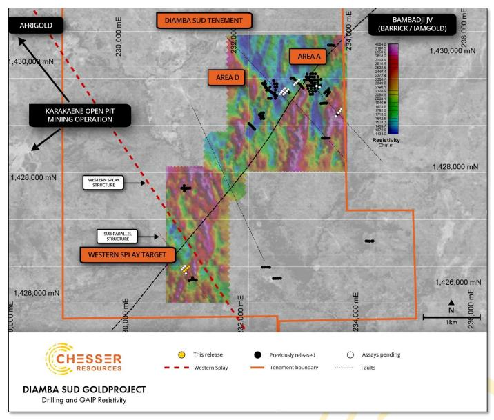
Figure 3: Diamba Sud Gold Project showing location of drilling for current results, assay results pending from Phase 4 drill program, resistivity from gradient array geophysics, interpreted structures and drilling targets (Area A, D and Western Splay)<sup>3</sup>.
