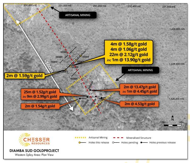
Figure 1: Results from initial Western Splay target area drilling. The structure appears to be a sub-parallel structure to the Western Splay structure based on geophysics. Historic drilling and artisanal activity indicate a potential strike length of 500m, open in both directions.<sup>2</sup>
