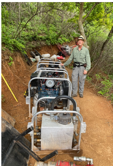
Photo 1: Hall Stewart next to the man-portable diamond core rig motors near the first drill pad at La Soledad, Copalquin.
