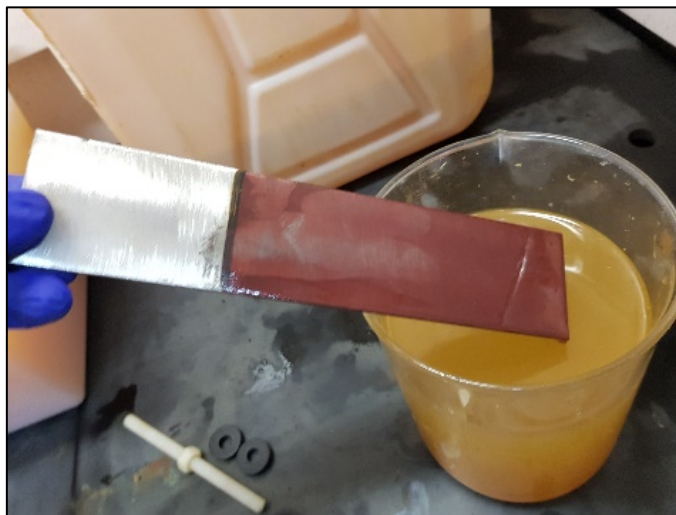
Figure 6: Image showing result of electrowinning test
