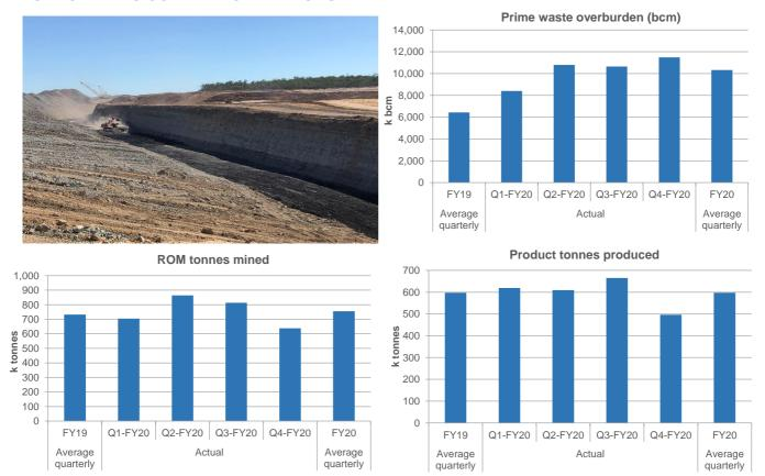
Stanmore achieved a record year for prime waste mining with 41.3Mbcm moved, driven by industry leading dragline performance of 17Mbcm (total) waste (nameplate capacity of 15Mbcm) and the commencement of the CAT6060 excavator in November 2019 moving 7.7Mbcm (13.2Mbcm annualised rate). This performance enabled ROM coal of 638kt to be mined in the quarter, resulting in a full year record of 3.02Mt coal mined.
