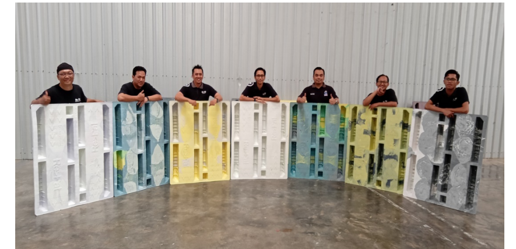
Picture of client trial where Dynapak's mixed waste was transformed into Re>Pal pallets using 100% mixed PP/ PE waste
