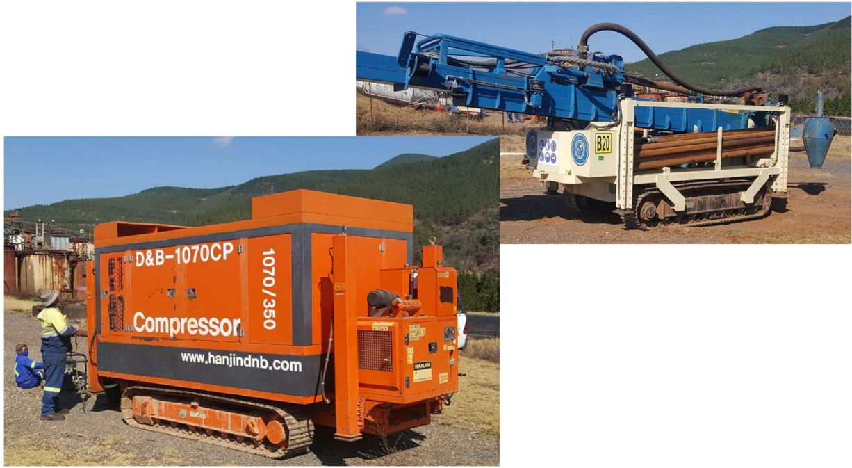
Figure 1: Track mounted reverse circulation drill rig and compressor on site at the Starter Theta Pit
