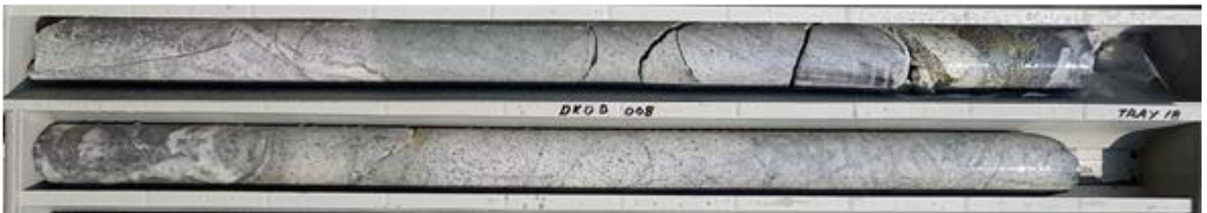
Photo 4 - DKDD008 ~64.9 to 65.3m ~40cm wide quartz-sulphide vein intercepted in the hanging wall of the projected underground exploited vein/lode.
