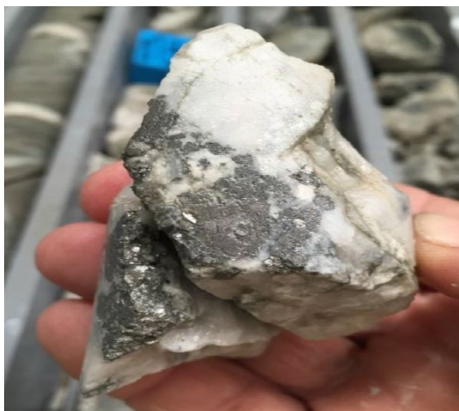
Photo 2 Drill core from hole CCD001 displaying mineralised quartz veining with arsenopyrite
