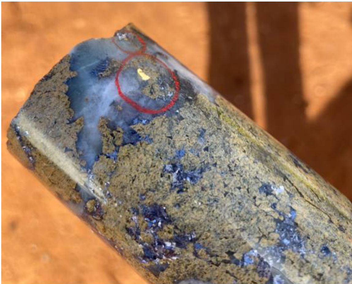
Figure 2. Drill core with very coarse-grained gold to 4mm (circled) associated with massive low-iron sphalerite (light brown), galena (metallic grey) and quartz (white) from FDD085. This sample is a part of a one metre interval grading 59.5% Pb+Zn and 137g/t Au.
